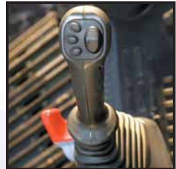
Joysticks with proportional control button for attachments
