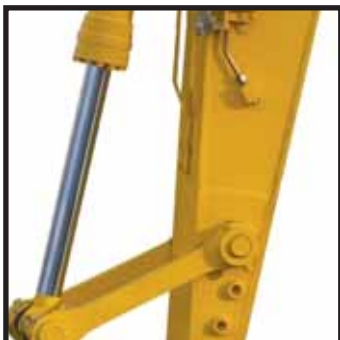
Quick-coupler piping standard
